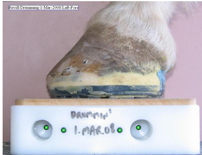
Lateral Photo: Metron prompts you to pick the four black markers on the block. Here, they are highlighted in green after they are picked.
